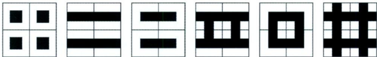
Figure 5. Generic urban forms, based on Martin and March. From left to right: pavilions, slabs, terraces, terrace-courts, pavilion-courts and courts
